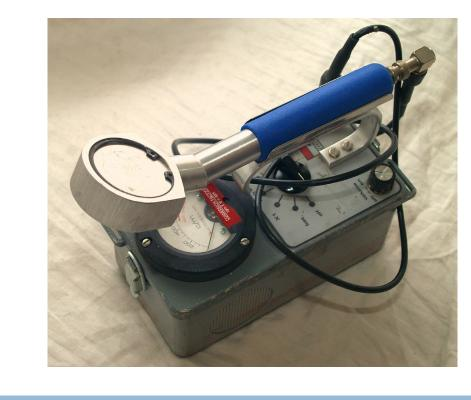
CPM-measuring field instruments have two parts: a probe that detects sources of radiation and a ratemeter, which connects to the probe. When the instrument detects a source of radiation, the ratemeter shows measurements of detected radiation in CPM.
